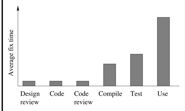
So we would like to have reasonably high quality components before testing and catch difficult defects early.
