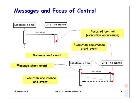
**Focus of control (execution occurrence)**: an execution occurrence (shown as tall, thin rectangle on a **lifeline**) represents the period during which an element is performing an operation. The top and the bottom of the of the rectangle are aligned with the **initiation** and the **completion time** respectively.
