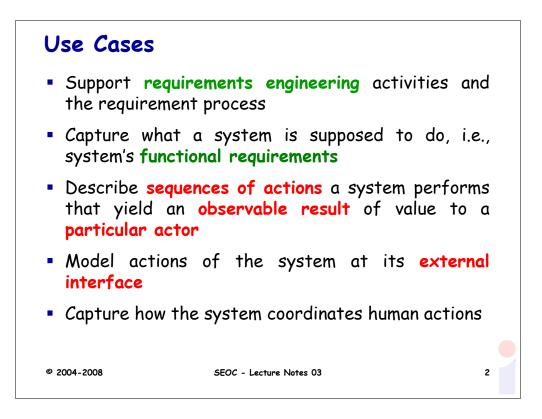
Use cases provide a high level view of the system. They capture to a certain extent system structures. Use case describe **sequences of actions** a **system performs** that yield **an observable result of value** to **a particular actor**.
