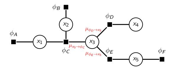
Message:  $\mu_{x_3 \to \phi_C}(x_3) = \tilde{\phi}_{54}(x_3) = \tilde{\phi}_4(x_3)\tilde{\phi}_5(x_3) = \mu_{\phi_D \to x_3}(x_3)\mu_{\phi_E \to x_3}(x_3)$
