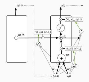
• Output gate: controls how much of each unit's activation is output by the hidden state – it allows the LSTM cell to keep information that is not relevant at the current time, but may be relevant later
