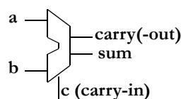
$$\text{sum} = \bar{a}\bar{b}.c + \bar{a}.b\bar{c} + a\bar{b}.\bar{c} + a.b.c$$
