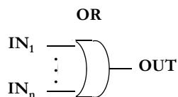
$$\text{OUT} = 1 \text{ if } \underline{\text{any}} \text{ } \text{IN}_i = 1$$
