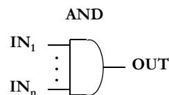
$$\text{OUT} = 1 \text{ if } \underline{\text{all}} \text{ } \text{IN}_i = 1$$
