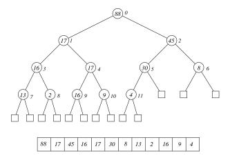
Direct mapping: *j*-th element of heap stored in index j - 1. Can use  $(2^i - 2) + j$  for index of *j*th element on level *i*. (depends on "Almost-complete" property).
