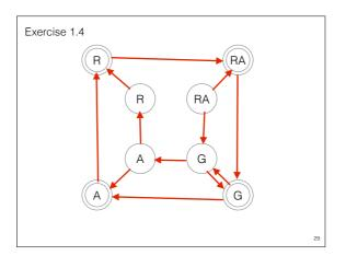
As discussed in the lecture, the diagram represents the beginnings of a refinement of our description of the traffic light controller. We model a sensor that detects a car ready to pass the light. For each state of the lights, (R, RA, G, A) we have two states, one (with a double circle) where there is a car, and the other, without a car, as before.
