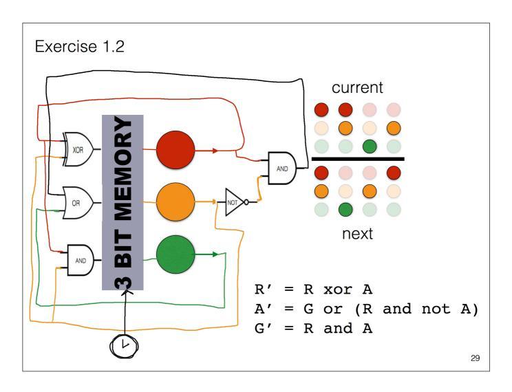
This implementation is based on a logical characterisation, for each light, of the set of current states such that the light is on in the next state. Check that the expression for A' gives the correct answer in each of the four cases.
