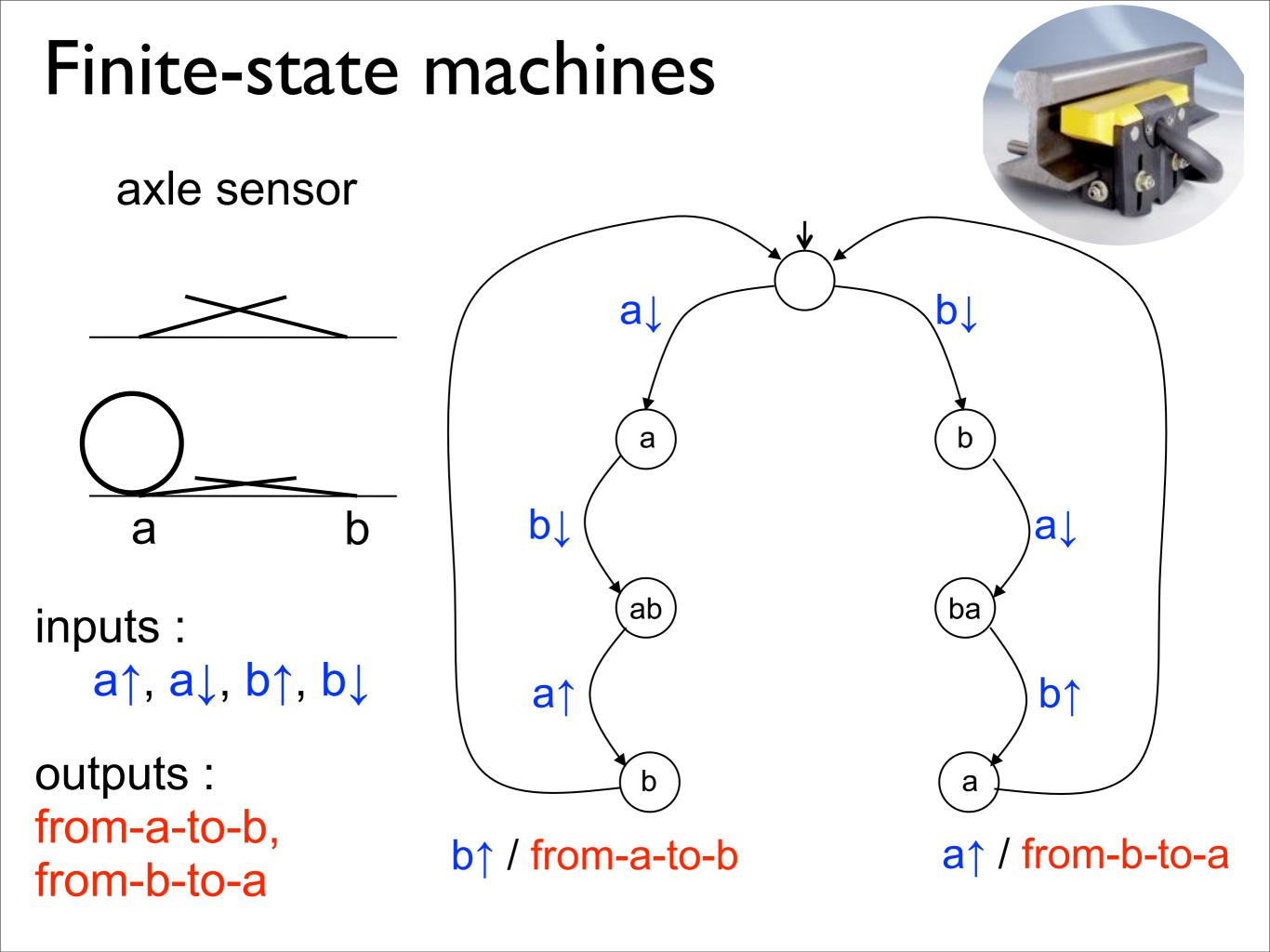
This is a finite state machine (or automaton).
