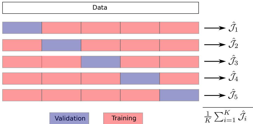
Figure 4.8: Sketch of K -fold cross-validation for K = 5 .
