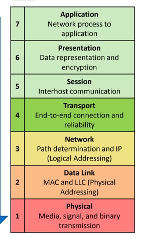
A firewall takes in network traffic and compares it to a set of rules. In order to do so it must first process several OSI levels to reach the data it needs.
