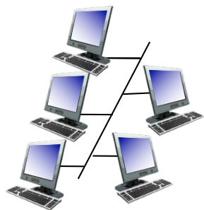
shared wire (e.g., cabled Ethernet)
