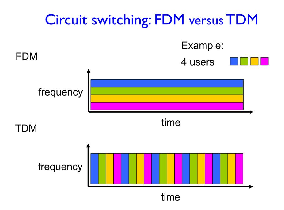
Packet switching versus circuit switching
