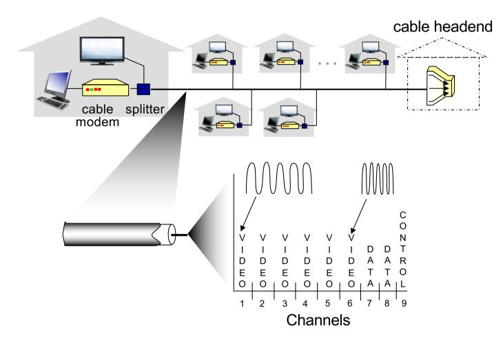
*frequency division multiplexing*: different channels transmitted in different frequency bands
