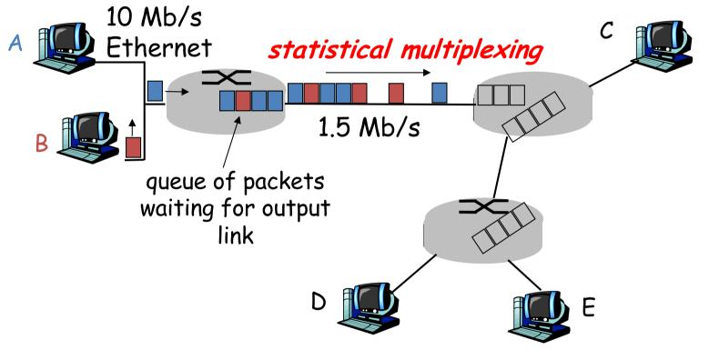
Sequence of A & B packets does not have fixed pattern **statistical multiplexing**.
