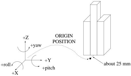
The position that the robot is at refers to the position of the gripper tip. The naming of the joints is:
