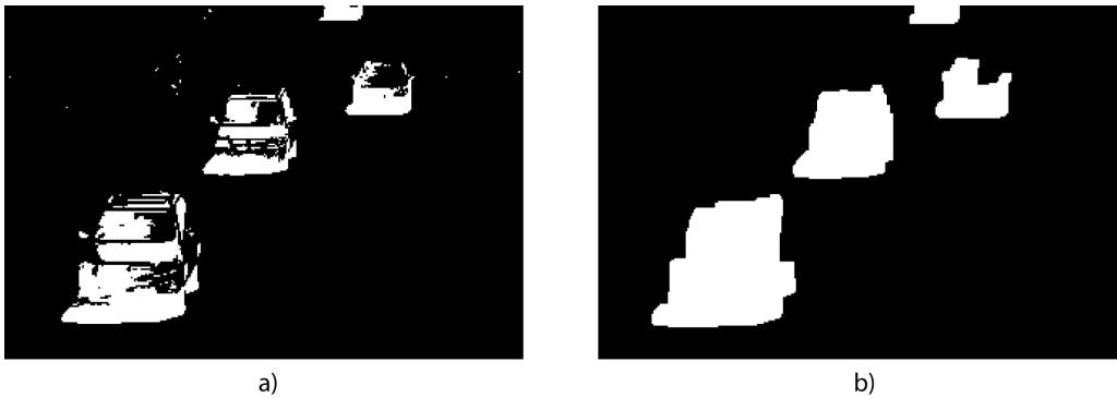
Figure 2: a) Background subtracted, b) Background subtraction method after refinement.
