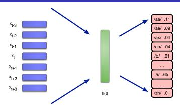
$$h_k = \sigma \left( \sum_{d=1}^{D} v_{kd} x_d + b_k \right)$$
