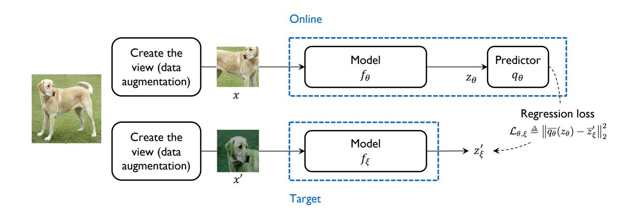
Iteratively train target network, parametrized as a moving average of online:
