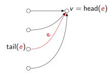
$$\alpha(v) = \sum_{e \in \text{in}(v)} p(X_e | W_e) \alpha(\text{tail}(e))$$
