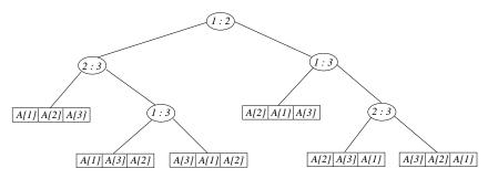
In insertion sort, when we get the result of a comparison, we often swap some elements of the array. In showing decision trees, we don't *implement* a swap. Our indices always refer to the *original* elements at that position in the array. To understand what I mean, draw the evolving array of INSERTIONSORT beside this decision tree.
