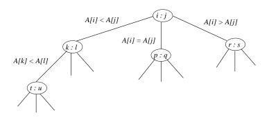
At each leaf of the tree the output of the algorithm on the corresponding execution branch will be displayed. Outputs of sorting algorithms correspond to permutations of the input array.
