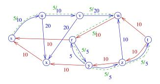
Now there is only one simple augmenting path -  $s \to u \to v \to w \to r \to y \to z \to t$ , with minimum residual capacity 5.
