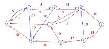
Residual network after adding 3rd flow, of value  $5 \Rightarrow$  total flow 25.
