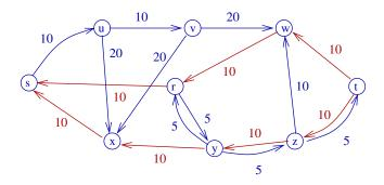
Residual network after adding flow from second augmenting path  $s \to x \to y \to z \to t$ , overall flow now 20.
