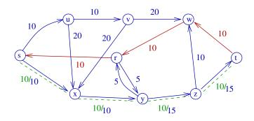
There is no longer any augmenting path of length  $\leq 3$ , and the only one of length 4 is  $s \to x \to y \to z \to t$ , which has a minimum capacity  $\min\{10, 10, 15, 15\}$ , ie 10.
