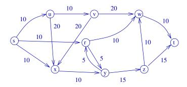
We will run Ford-Fulkerson (with the Edmonds-Karp heuristic) on this network. This is interesting because we will see the "back-edges" being used to "undo" part of an previous augmenting path.
