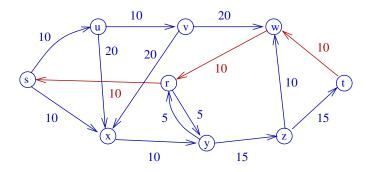
Residual network after adding first flow of value 10 along  $s \to r \to w \to t$ . The newly-created "back-edges" are shown in red.
