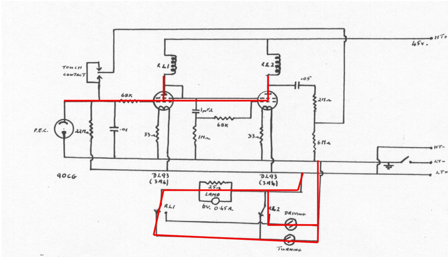
Strong light: switches relay 1, turning motor in series with lamp; turns smoothly away from light.
