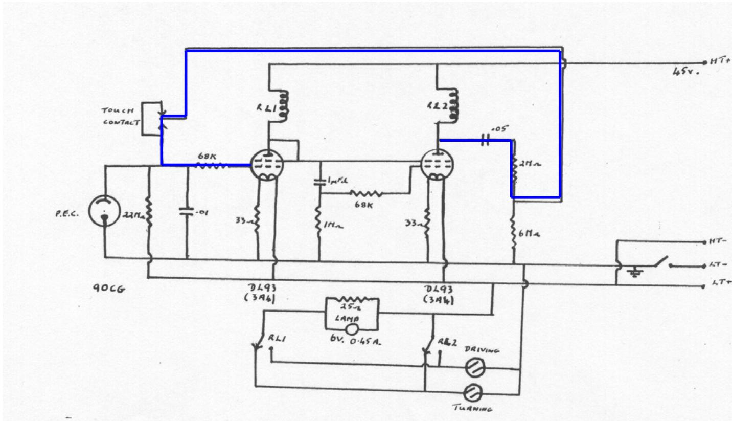
Shell collision: closes touch contact, output of amplifier 2 becomes input to amplifier 1; produces oscillator.
