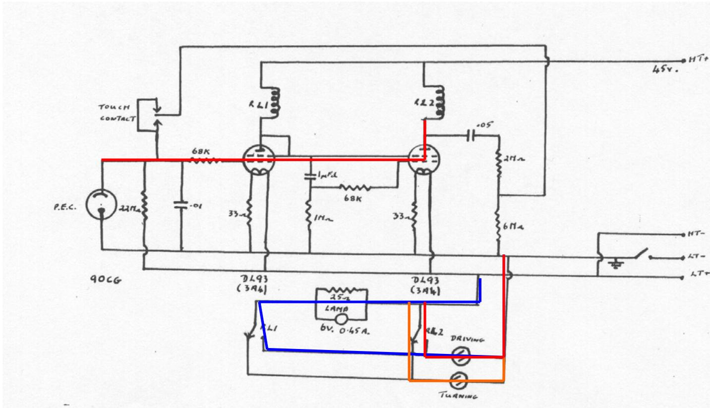
Starts with: drive motor in series with lamp and turning motor full on; get cycloid movement that scans for light.
