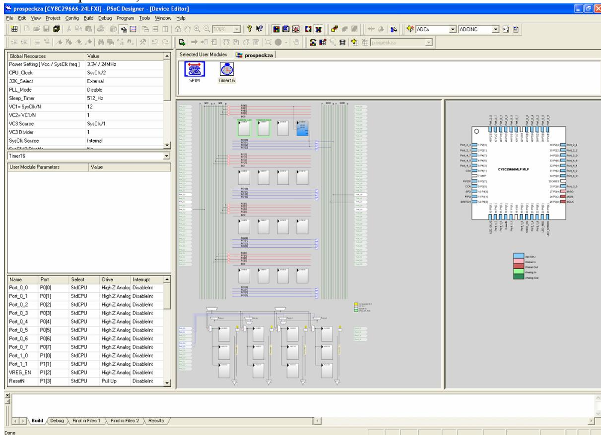
This screen is where you place the modules into their blocks and setup the interconnections. The parameters of the modules are also modified here (which can be changed using software as well). You would see 2 sets of blocks. The top 4 rows are digital blocks and the last 3 rows are analog blocks. For more details of the blocks and their possible connections to other blocks, please read the CY8C29666 manual.
