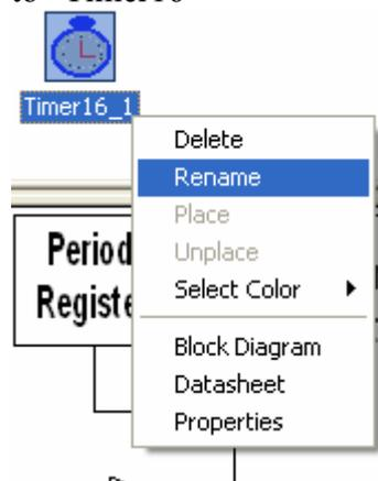
That's it. You have just selected a 16-bit timer into the ProSpeckz configuration. The next step is to configure the timer.
