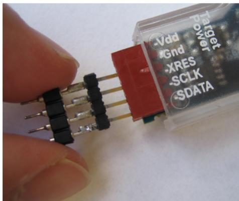
Next, connect the MiniProg to the ProSpeckz as shown below. Take note of the orientation of the MiniProg.
