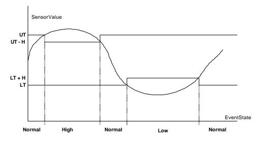
The hysteresis is used to limit spurious state transitions when the sensor value is close to a threshold.
