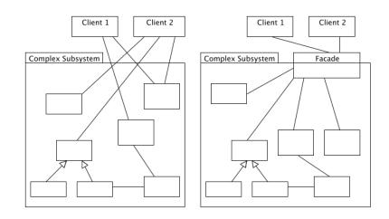
Image: http://best-practice-software-engineering.ifs.tuwien.ac. at/patterns/facade.html **Common problem:** you have roughly separated your classes into two packages, but there are several dependencies of classes in package A on classes in package B. It becomes hard to work out what the effect of a change in package B will be, and developers who want to use the services of package B have to understand the detail of what's inside it.
