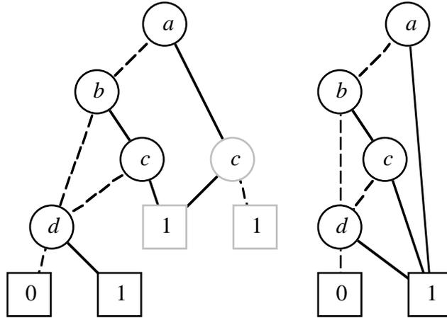
Figure 8: **Result Generation for APPLY operation.** The recursive calling structure naturally leads to an unreduced graph (left). By applying reduction rules at the end of each recursive call, the reduced graph is generated directly (right).
