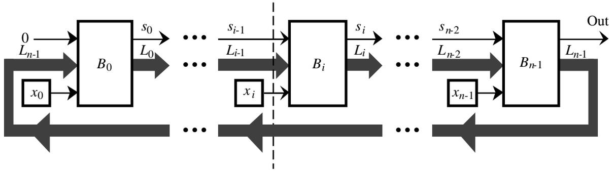
Figure 5: **Linear Arrangement of Within- $K$  Ring Circuit.** As shown by the dashed line, the circuit has forward cross section  $2 + \lfloor \log_2 K \rfloor$  and reverse cross section  $\lfloor \log_2 K \rfloor$ .
