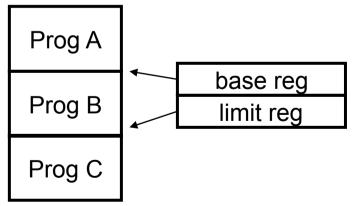
base and limit registers are loaded by OS before starting program
