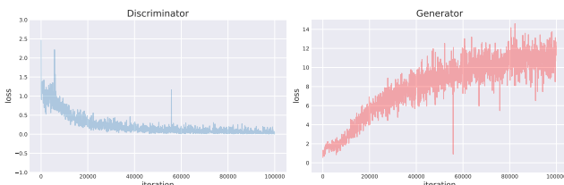
Figure 7. Discriminator and Generator losses plotted over training iterations for a successful experiment with our conditional GAN architecture.
