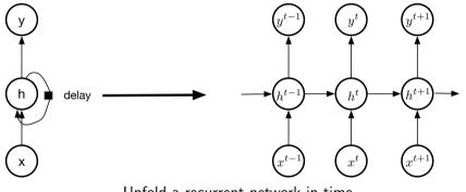
Unfold a recurrent network in time
