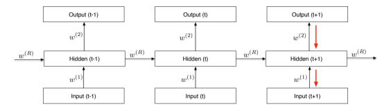
• View an RNN for a sequence of T inputs as a T-layer network with shared weights
