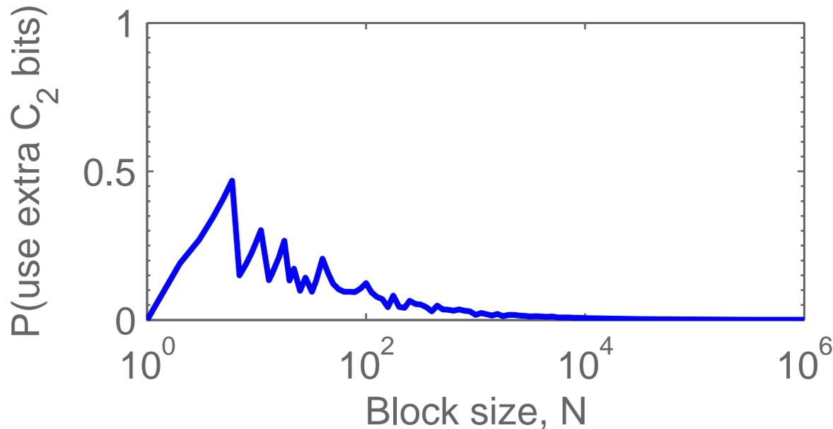
*With high probability we can compress a large- $N$  block into a fixed number of bits. Empirically  $\approx 0.47 N$  for  $p=0.1$ .*
