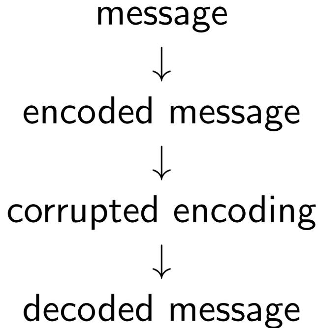
Rather than cooling a system, or increasing power, we send more robust encodings over the existing channel
