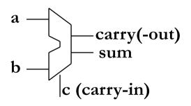
$$sum = \overline{a.b.c} + \overline{a.b.c} + a.\overline{b.c} + a.b.c$$
