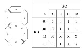
(b) The Karnaugh map is filled in from the (a) column.X represents an unspecified output – your logic may produce 0 or 1.What is the CNF required to drive the (a) segment?
