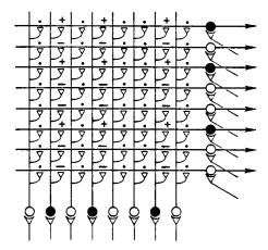
Active input pattern and corresponding output (indicated with + and -).
