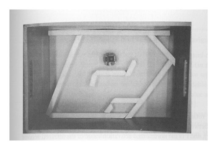
• Eight IR sensor input units, feed-forward to two motor output units with recurrent connections
