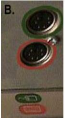
(ii) B provides color coding to associate the connectors with the labels
