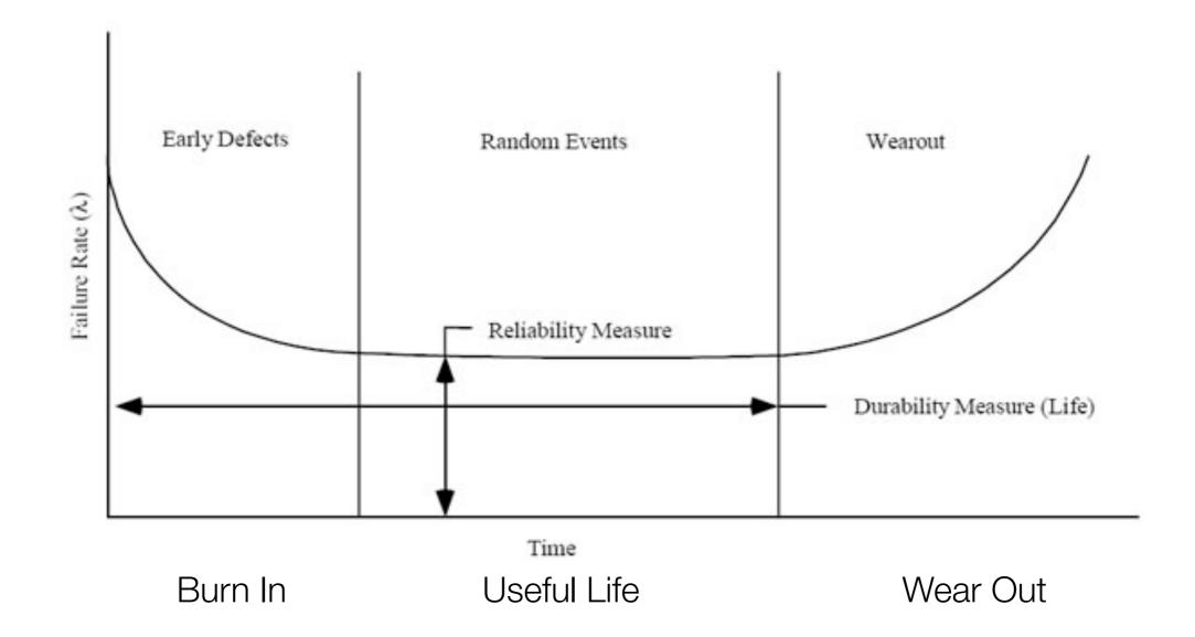
During useful life, components exhibit a constant failure rate  $\lambda.$  Reliability of a device can be modelled using an exponential distribution  $R(t)=e^{-\lambda t}$
