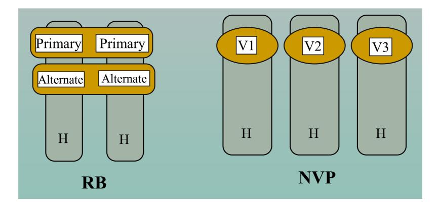
RB Scheme comprises of three elements: A primary module to execute critical software functions. Acceptance test for the output of primary module. Alternate modules perform the same functions as of primary.
