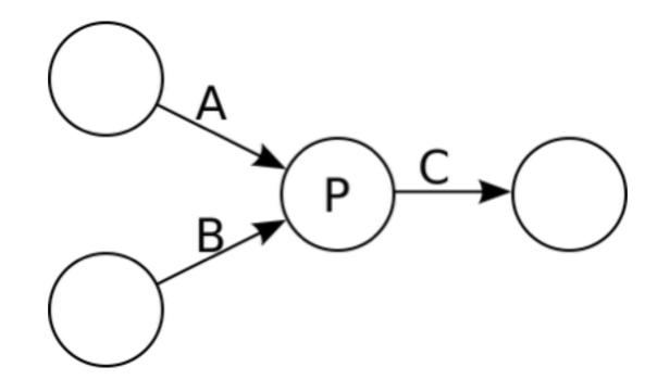
A Kahn process network of three processes without feedback communication. Edges A, B and C are communication channels. One of the processes is named process P.
