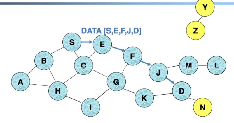
When node S sends a data packet to D, the entire route is included in the packet header, hence the name source routing
