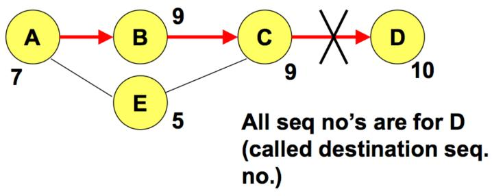
A does not reply, since its sequence no. is less than that of C
