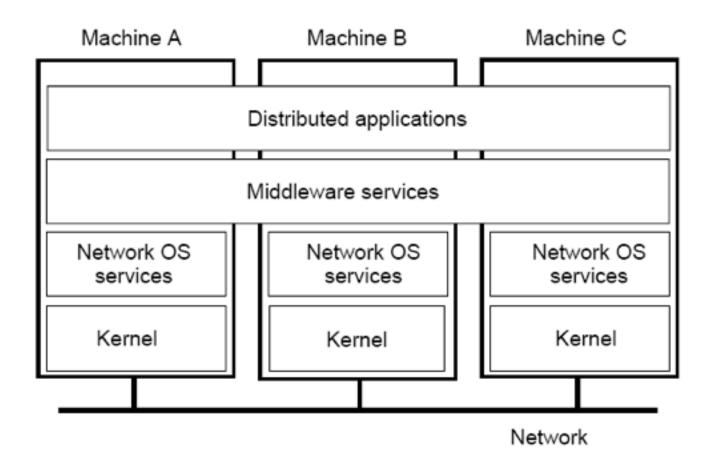
Fig. 1-22. General structure of a distributed system as middleware.
