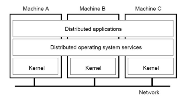
Fig. 1-14. General structure of a multicomputer operating system.
