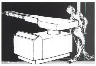
A neighboring employee discovered the victim pinned between the right rear of the robot and a safety pole in a slumped but upright position. The victim died five days later in the hospital.
