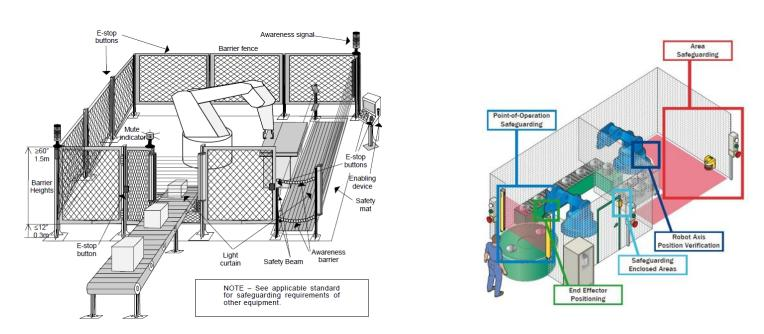
**Deployed robot safety systems**
