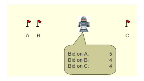
Each robot bids on a target the increase in minimal path cost it needs from its current location to visit all of the targets it has won if it wins the target (BidSumPath).
