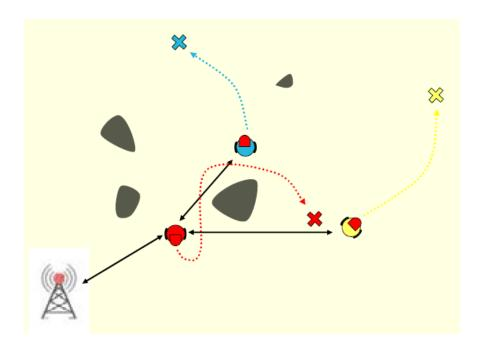
The red robot sends blue a counter offer of this joint plan to the blue robot and requests a bid from the blue robot. Although the path is long, blue's bid will be less costly because it will have communication with the tower. This path will be adopted by the two robots.
