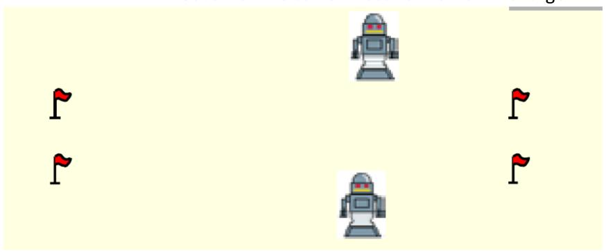
Each robot bids on a target the minimal path cost it needs from its current location to visit the target.
