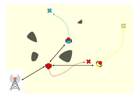
The blue robot proposes this joint plan to the red robot and requests a bid from the red robot for its participation. Red's bid will be too expensive because the proposed plan causes LOS loss between red and yellow.
