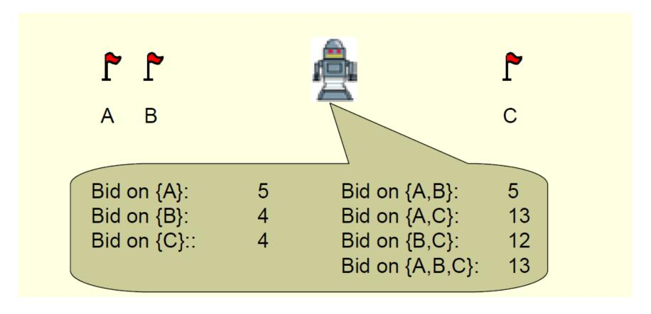
Each robot bids on a bundle the minimal path cost it needs from its current location to visit all targets that the bundle contains.
