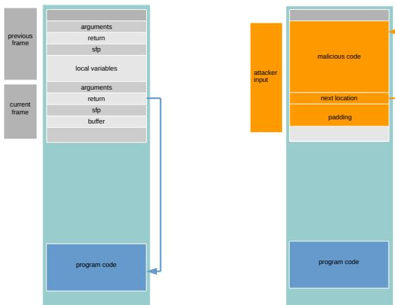
A buffer overflow can change the flow of execution of the program.
