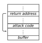
The malicious argument overwrites all of the space allocated for the buffer, all the way to the return address location. This is altered to point back into the stack, somewhere in a "landing pad" of NOPs before the attack code (the "egg"). Typically the attack code executes a shell.
