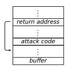
The malicious argument overwrites all of the space allocated for the buffer, all the way to the return address location. This is altered to point back into the stack, somewhere in a "landing pad" of NOPs before the attack code (the "egg"). Typically the attack code executes a shell.
