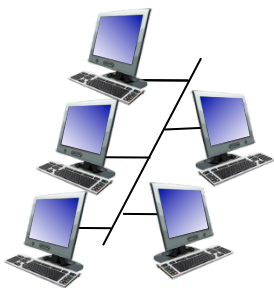
shared wire (e.g., cabled Ethernet)
