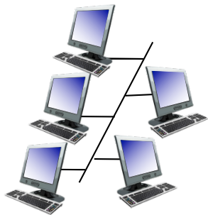
shared wire (e.g., cabled Ethernet)
