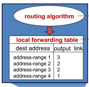
routing algorithm determines end-end-path through network
