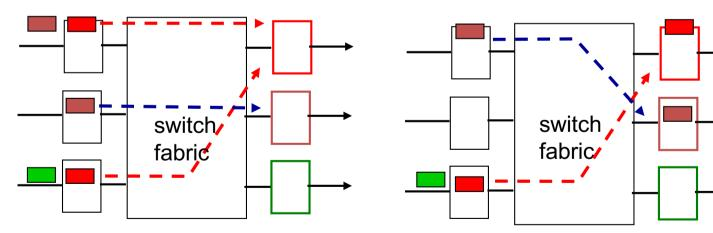
output port contention: only one red datagram can be transferred. *lower red packet is blocked*  one packet time later: green packet experiences HOL blocking
