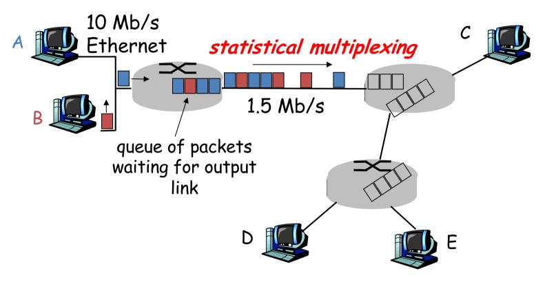
Sequence of A & B packets does not have fixed pattern **statistical multiplexing**.
