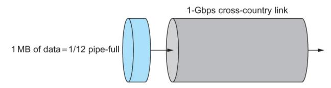
A 1-MB file would fill the 1-Mbps link 80 times, but only fill the 1-Gbps link 1/12 of one time
