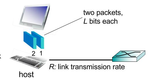
transmission delay time needed to transmit
