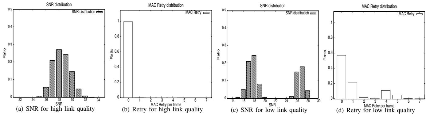
Fig. 4. Retry and SNR distribution at the receiver
