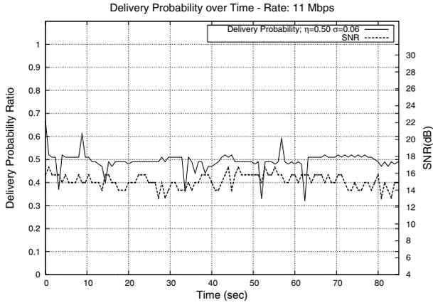
Fig. 1. DPR-RX and link quality for a selected link - 0.8 sec windowing
